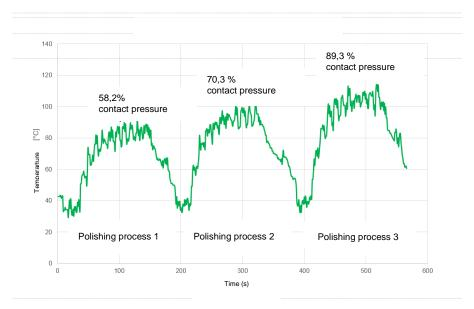
Figure 1 Temperature development in the robot cell during three polishing cycles with 10 passes each and different contact pressures
