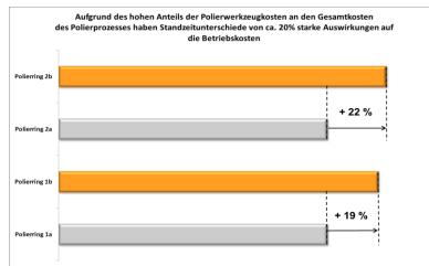
Fig. 3: Differences in service life for the tested polishing wheels
